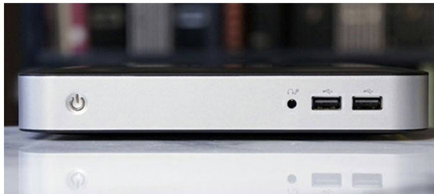
The front edge has a power button, power jack and two USB 2.0 ports.
