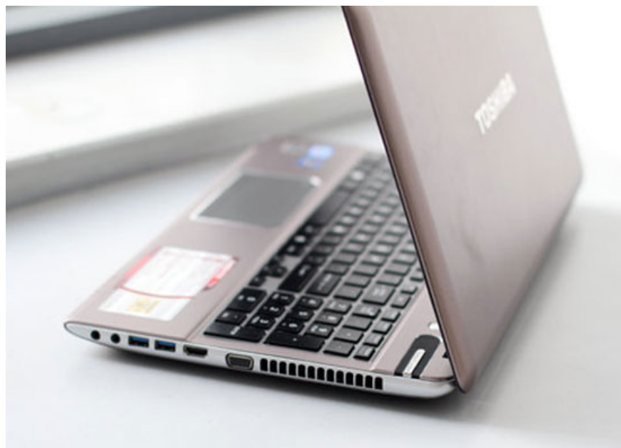
Next to the machine is the heat exit slot, USB 3.0, HDMI and headphone jack, microphone.
