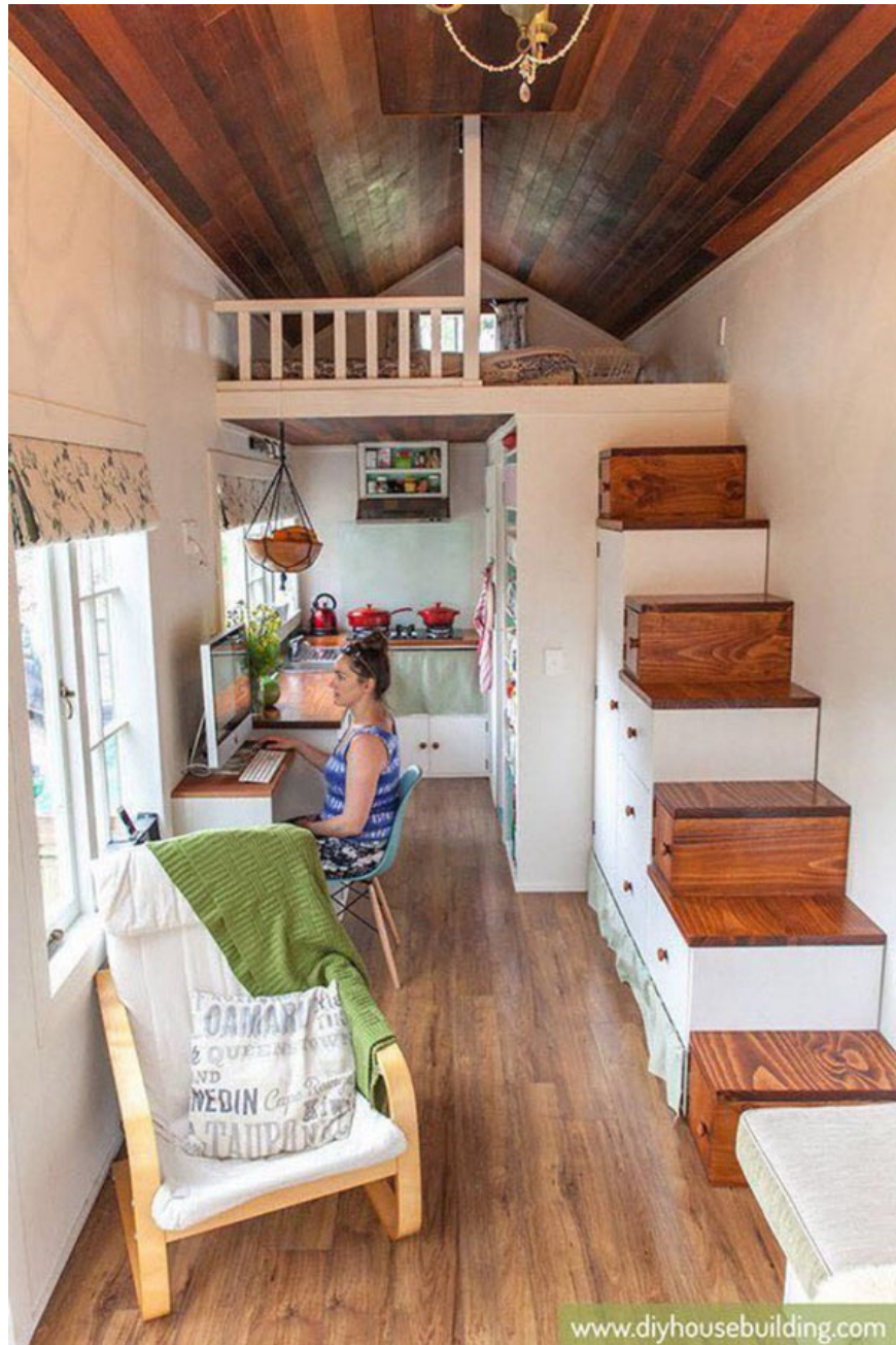
The super-small house still has enough functions thanks to the mezzanine that creates a private bedroom above and the cleverly designed storage system on the steps.
